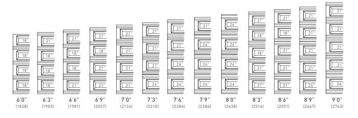
MEASUREMENTS: 18" = 457 mm 21" = 533 mm 24" = 610 mm \*Please note that the Martin Standard and the Cornerstone tongue and groove joint 8' (2438) vs 4 sections vs 5 section for the 8' Safety Joint Cornerstone.
